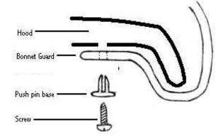
**3.** Fit the plastic "W" clips to the 4 holes at the outer edge of the Bonnet Guard. Apply the supplied rectangular pieces of anti-abrasive tape on edge of bonnet where plastic fastening "W" clips secure the Bonnet Guard.
