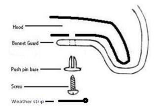
**5.** Apply the anti-abrasive tape on edge of bonnet where plastic fastening clip secures the Bonnet Guard near the fenders. Use the supplied
