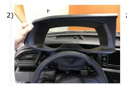
2) Removing the instrument panel frame.
