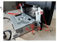
7 Screw the both brackets with 6 screws 'A' (3 on each side) to the main unit of Alpine Halo.
