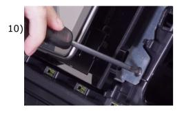
10) Screw the radio block into the dashboard using 4 screws 'B' (2 on each side), then replace the OEM radio frame. Attach the Alpine display to the assembled radio block in the dashboard and fix it.
