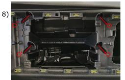
8 Place the radio block in the dashboard and mark the 4 holes.
