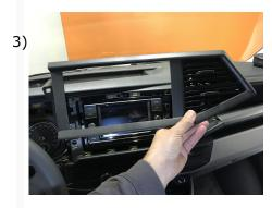
3) Removing the radio frame.
