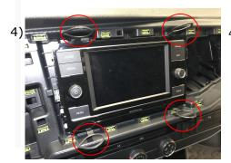
4) Removing OEM radios with Volkswagen keys.
