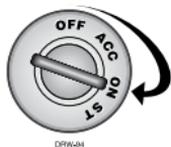
To disable the optional Failsafe Starter Kill, turn the ignition to the ON position. Press and release the Valet switch one time within 10 seconds. The status LED will stop flashing and the vehicle should start. If the vehicle does not start, you may have waited too long; turn the ignition off and repeat the process.
