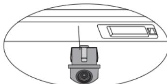
Pass the cable through the hole and press the camera and seal into the hole.
