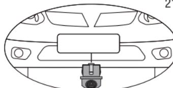
Lay the cable and connect it according to the description given on the next page. Then reinstall the bracket. In variant 2, you may have to Depending on the installation location (front or rear), two cable loops are cut. Otherwise the image will be displayed incorrectly. Please check this setting with the help of a monitor before final assembly.
