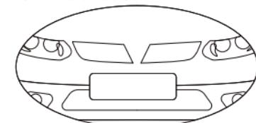
2. Install the KCX401 e.g. under the license plate in the front of the vehicle. To do this, drill an 21 mm hole.
