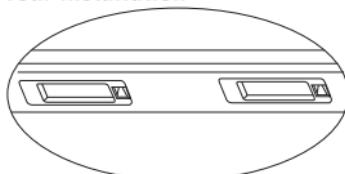
1. Install the KCX401 into your license plate light mount. To do this, dismantle the bracket and drill an 21 mm hole.
