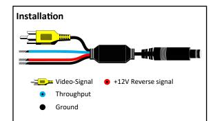
**Note:** If the camera is powered by reverse gear lamp signal, we recommend to install a relay between the power supply of the reverse signal and the power supply of the camera, to ensure a stable and uninterrupted power supply and to avoid unwanted errors in the vehicle computer.
