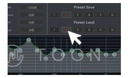
3. Select Preset Load slot #2 to display the DSP audio file settings stored in Preset Save slot #2
