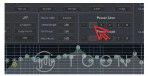
**CAUTION** Selecting a different Preset Load slot prior to selecting the Preset Save slot will result in the loss of the loaded DSP file.
