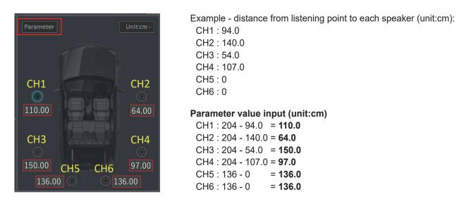
\* Time alignment parameters are automatically adjusted to the DSP optimized values when the screen is refreshed. E.g. Entered value of 10.0cm will automatically be adjusted to 9.860cm. The automatic adjustment occurs when selecting a different channel, changing alignment setting, changing the units etc.
