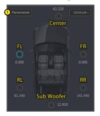
The listening area is determined by a imaginary circle of radius 204cm (80.315 in.), with its center at the listening point. The listening point is typically the driver's head position.
