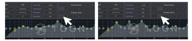
Result: Preset Load slot #1 contains the original DSP audio file and Preset Load slot #2 contains the modified DSP audio file
