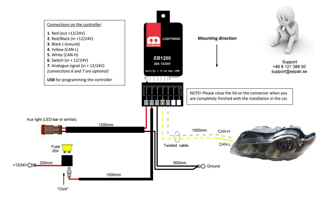
NOTE! White (CAN-H) and yellow (CAN-L) twisted cable = Digital signals in.
