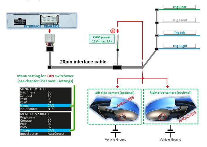
Power supply for side-cameras should be connected to green wire CAM power 12V (max 3A) of 20pin interface cable, as this cable is only powered during camera activation (some cameras are not continuously current stable).
