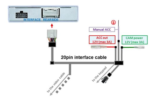
1 Connect purple wire Manual ACC of 20pin interface cable to +12V S-contact terminal 86s or ACC terminal 15r of vehicle (e.g., cigarette lighter, glove compartment illumination).
