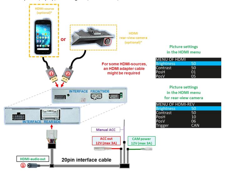
If an optional HDMI video-source (e.g., smartphone, laptop, etc.) is connected to the HDMI-input\*, the video shown on the display of the HDMI-source will be mirrored on the vehicle monitor. The video-signal from display-free sources (e.g., streaming stick, DVD-Player, DVB-T2 Tuner, etc.) will be displayed on the vehicle monitor. The power supply for the video-source can be taken from red wire ACC out 12V (max 3A).
