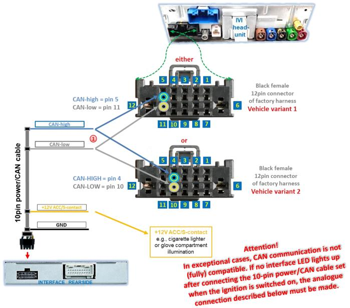
Connect blue CAN-high wire and grey CAN-low wire of 10pin power/CAN cable to corresponding chambers of black female 12pin connector of vehicle harness. There are two known vehicle pin definition variants displayed above.
