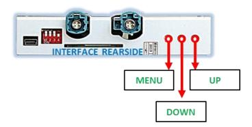
The picture settings are adjustable by the 3 push-buttons at the rear-side of the video-interface. Press the MENU button to open the OSD settings menu or to switch to the next menu item. Press UP and DOWN to change the selected value. The buttons are placed inside in the housing to avoid accidental changes during or after the installation. Picture settings must be done separately for all video inputs while the corresponding input is selected and visible on the monitor.
