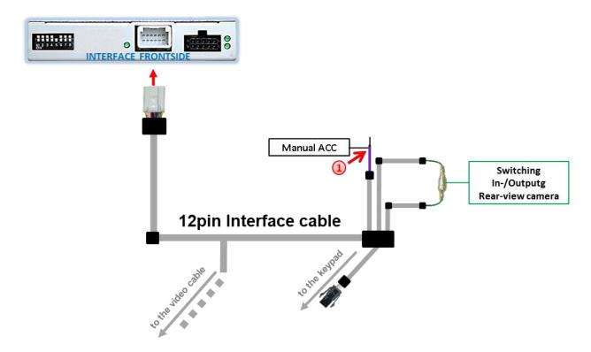
1 If, after connecting the PNP harness, no interface LED lightens up while the ignition is turned on, the purple coloured wire Manual ACC of the 12pin interface cable has to be connected additionately to ACC or S-contact terminal 86s +12V (e.g. glove compartment illumination).
