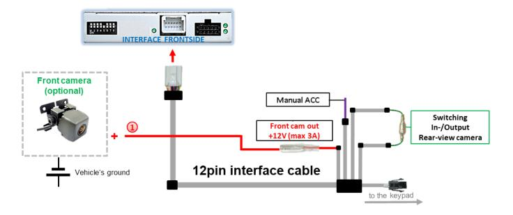
The red power supply output Front cam out +12V (max 3A) can be used to power a front camera. If Dip 1 is set to ON (black 8 dips), the power supply output gives +12V (max 3A) when reverse gear is engaged and additionally for 10 seconds after the reverse gear has been disengaged.
