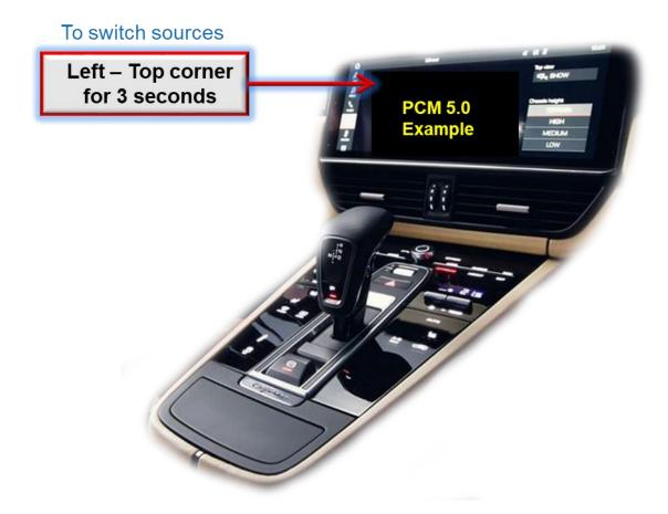
Long press the left top corner of the factory touch screen to switch the video-source.
