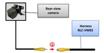
Connect the video RCA of the after-market rear-view camera to female RCA connector of harness RLC-VW03.
