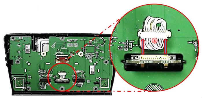
3 Disconnect the female 12pin connector from its 12pin SD card connector (keep connected at mainboard).
