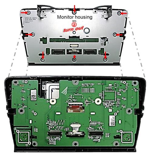
2 Turn out the 8 screws (red arrows) at the rear-side of the monitor and remove the metal sheet to set free the mainboard's ribbon cable base with the factory picture signal cable.
