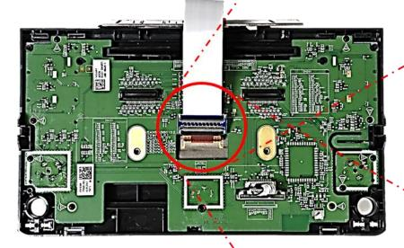
3 To avoid any kind of vibration-caused short circuits After the connection, it's necessary to isolate both sides of the merger with some kind of smooth issue tape as shown in the picture beside.
