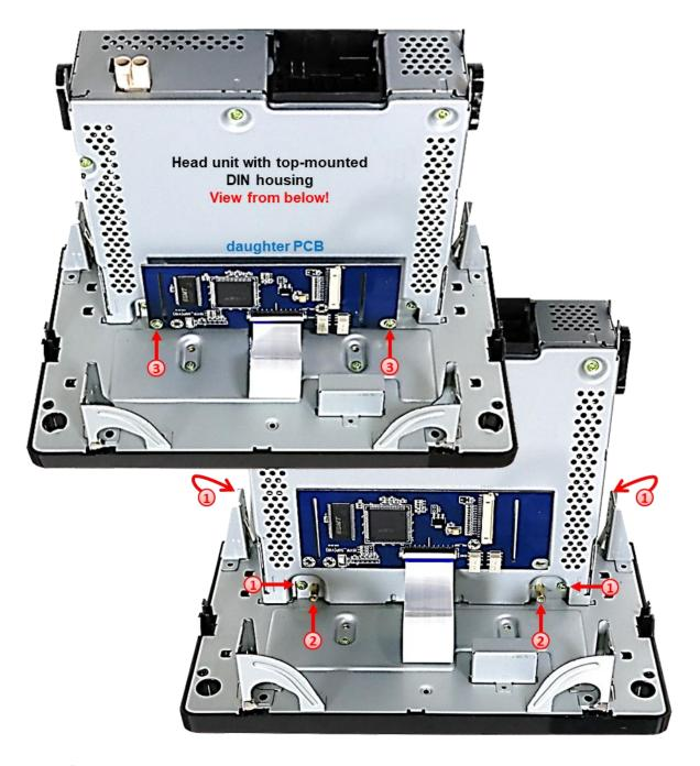
Carefully, plug the head unit into the monitor again and fix it with the 4 screws on its top and its bottom.
