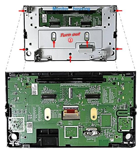
2 Turn out the 7 screws (red arrows) at the rear side of the monitor and remove the metal sheet to set free the mainboard's ribbon cable base with the factory picture signal cable.
