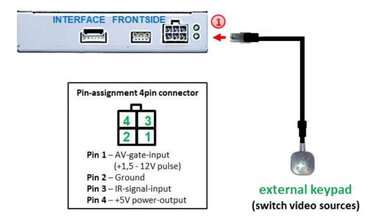
Connect the 4pin female connector of the external keypad to the male 4pin connector of the video interface.
