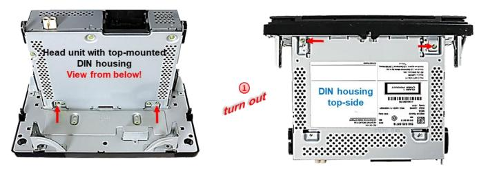
1 Turn out both screws at the **outer** side of the top part of the head unit (red arrows) and both screws at the bottom part of the head unit (red arrows). Remove the head unit from the monitor and lay it aside.
