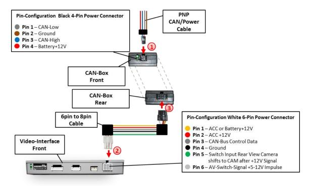
Connect the black female 4pin Micro-Fit connector of the PNP Can/Power Cable to the 4pin Micro-Fit connector of the CAN-box.
