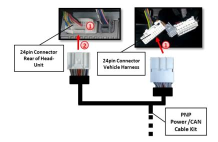
Disconnect the 24pin connector of the vehicle harness at the rear of Monitor and connect it to the 24pin Connector of PNP Power/CAN Cable Kit.
