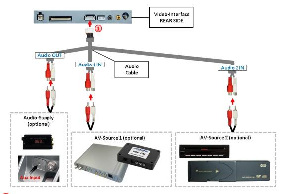
Connect the female 7pin connector of the audio cable to the male 7pin connector of the video-interface.
