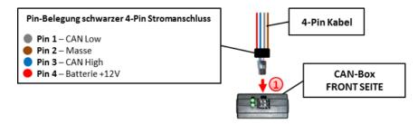
Connect the stripped ends of the 4pin cable to Ground, Battery +12V, CAN high- and low, of the vehicle's monitor harness, without cutting them.
