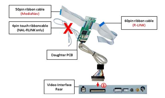
Connect the female 20pin connector of the daughter PCB to the male20pin connector of the 20pin cable and connect the second male 20pin connector opposite the cable to the female 20pin connector of the interface. Take care for installing the cable in the right direction as both connectors are identical. (Take notice of the wire's caption "MONITOR SIDE" and "BOX SIDE"
