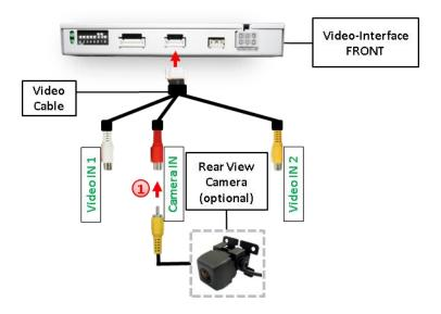
Connect the video-RCA of the after-market rear-view camera (NTSC only) to the female RCA port of the video-interface which is labelled as CAM.
