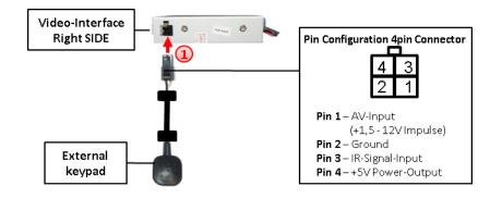
Connect the female 4pin connector of the keypad to the male 4pin connector of the video-interface.
