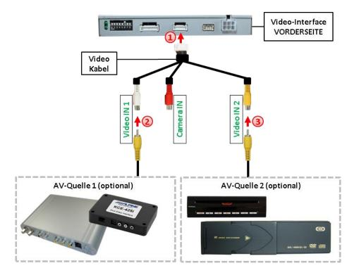
Connect 6pin male connector of video cable to female 6pin connector of videointerface
