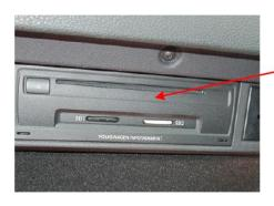
Remove the original radio, disconnect Quadlockconnector and connect Yharness
