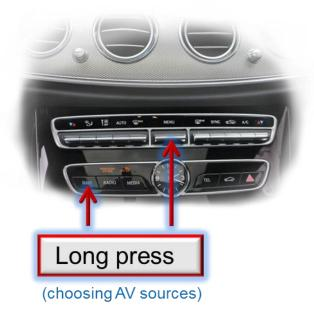
A short press of the NAVI button or the Menu button switches the input from factory mode to the inserted video sources.
