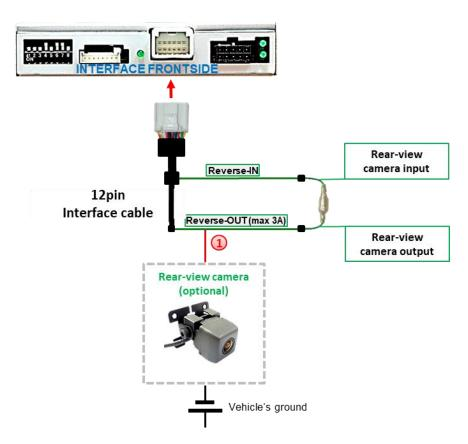
1 Additionally, the +12V (max. 3A) power supply for the rear-view camera can be taken from the green wire of the 12pin interface cable.
