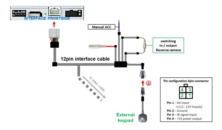
Onnect the female 4pin connector of the keypad to the male 4pin connector of the 12pin interface cable.
