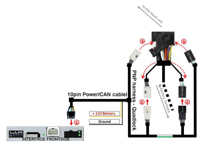
Connect the female 10pin connector of the 10pin Power / CAN cable to the 10pin connector of the video interface.
