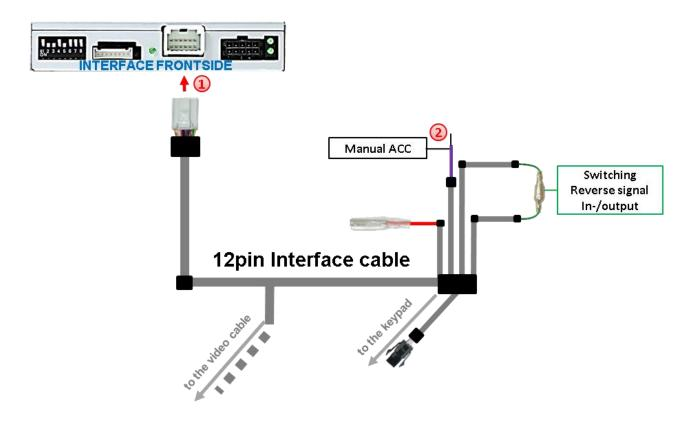
1 Connect the enclosed 12pin interface cable's female 12pin connector to the male 12pin connector of the video interface.
