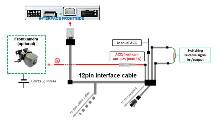
1 The red power supply output ACC/front cam out 12V (max 3A) can be used to power a front camera. If Dip 1 is set to ON (of the black 8 dips), the power supply output supplies +12V (max 3A) when the reverse gear is engaged and additionally 10 seconds delay after reverse gear is disengaged.
