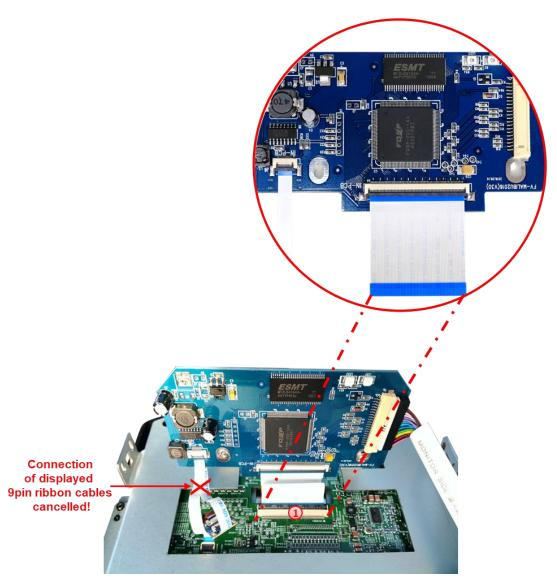
Onnect the daughter PCB's pre-assembeled 66pin ribbon cable "IN PCB" to the previously become free ribbon cable base of the monitor mainboard (heed the following warning notes!).
