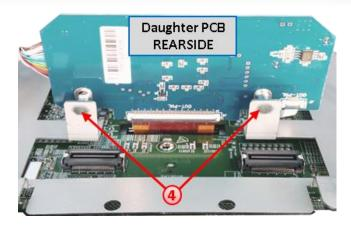
4 After connecting the ribbon cables, the daughter PCB has to be fixed with its rearside at the exchange retaining plate by using the enclosed 2 shorter screws.
