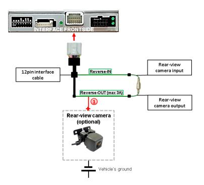
The 12 V power supply for the rear-view camera (max 3A) has to be taken from the green wire of the 12pin interface cable to avoid an unnecessary, permanent power supply to the camera electronic.
