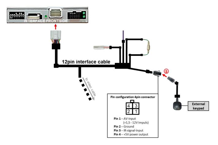
1 Connect the keypad's female 4pin connector to the video-interface's male 4pin connector.
