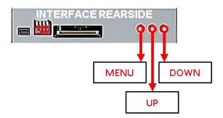
The picture settings are adjusted by the 3 buttons on the video-interface. Press the MENU button to open the OSD settings menu. To switch to the next menu item, pressing UP and DOWN will change the selected value. The buttons are embedded in the housing to avoid accidental changes during or after installation. The picture settings have to be done separately for AV1 and AV2 while the corresponding input is selected and visible on the monitor.
