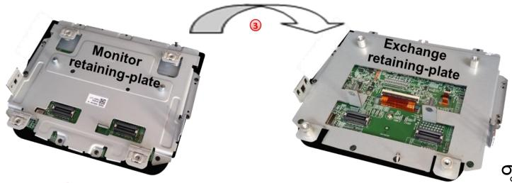
Remove the Original monitor retaining plate and replace it with the exchange retaining-plate by using the original screws. عae ر
