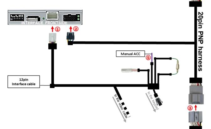
4 Connect the female 20pin connector of the 20pin PNP harness to the male 20pin connector of the head-unit.
