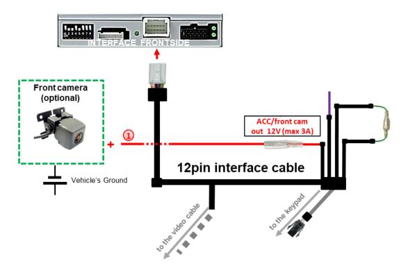
1 The red power supply output ACC/front cam out 12V (max 3A) can be used to power a front camera. If Dip 1 is set to ON (of the black 8 dips), the power supply output gives +12V (max 3A) when reverse gear is engaged incl. 10 seconds delay after reverse gear is disengaged.
