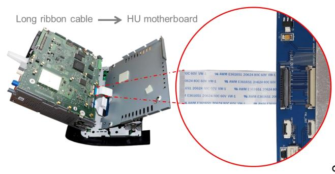
After a check of the perfect ribbon cable connection, in reverse order fold back and clip in the head-unit housing to the head-unit control panel and fix the exchange housing base plate to the head-unit's housing.
