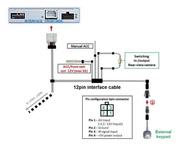
Onnect the keypad's female 4pin connector to the 12pin interface cable's male 4pin connector.
