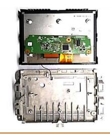
Remove the metal bracket behind the screen as shown above.
