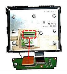
Carefully clip out and disconnect the PCB board's 68pin ribbon cable from its ribbon cable base.
