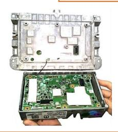
Carefully separate the rear-side from the monitor. Take care not to break the coaxial wire in between.
