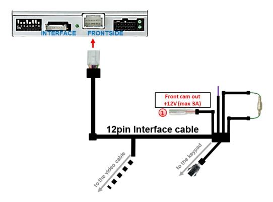
The red power supply output Front cam out +12V (max 3A) can be used to power a front cam with dip switch 1 (of the black 8 dips) to ON.
