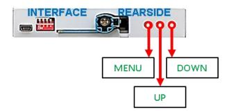
The picture settings are adjustable by the 3 push-buttons of the daughjter PCB's menu keypad. Press the 1. button to open the OSD settings menu or to switch to the next menu item. By pressing the other both push buttons the selected value will be changed. To avoid accidental changes during or after the installation, we recommend to disconnect the keypad from the pushbutton cable after the adjustments are done. Adjustments have to be done, while the selected input is visible on the monitor.
