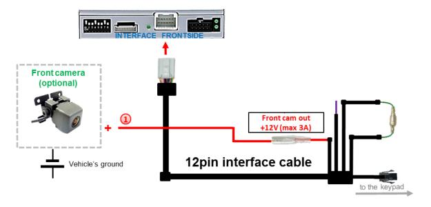
1 The red power supply output Front cam out 12V (max 3A) can be used to power a front camera. If Dip 1 is set to ON (black 8 dips), the power supply output gives +12V (max 3A) when reverse gear is engaged incl. 10 seconds delay after reverse gear is disengaged.
