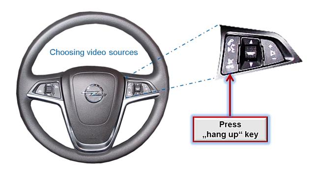
To switch the interface's activated video sources, the factory infotainment buttons can be used.
