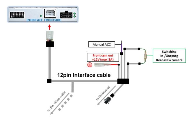
The red power supply output Front cam out +12V (max 3A) can be used to power an external source and has a different assignment, depending on the position of dip switch 1 (of 8 dips):
