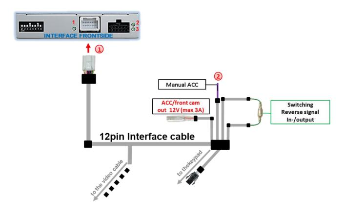
1 Connect the red wire ACC-OUT and the purple coloured wire Manual ACC of the 12pin interface cable to +12V ACC power supply.
