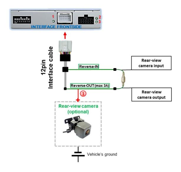
The 12 V power supply for the rear-view camera (max 3A) has to be taken from the 12pin interface cabl's green wire "Reverse-OUT" to avoid an unnecessary, permanent power supply to the camera electronic.
