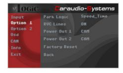
Exception: Connect the yellow/red wire to the right analogue blinker signal and the yellow/green wire to the left analogue blinker signal of harness V6C-NAC01 (triggered +12V blinker power) and make the menu setting - Option 2 / Cam Trigger - "Analogue", if the system doesn't switch to the aftermarket side view camera automatically after the described OSD-setup (Option 2 / Cam Trigger - "CAN", see next chapter).
