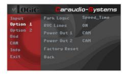
Exception: Connect the yellow/red wire to the right analogue blinker signal and the yellow/green wire to the left analogue blinker signal of harness V6C-NAC01 (triggered +12V blinker power) and make the menu setting - Option 2 / Cam Trigger - "Analogue", if the system doesn't switch to the aftermarket wide view front camera automatically after the described OSD-setup (Option 2 / Cam Trigger - "CAN", see next chapter).
