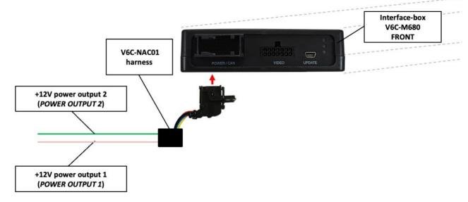
You can configure the both +12V trigger outputs separately. The pink wire is (*POWER OUTPUT 1*) is Power Out 1 and the green wire is (*POWER OUTPUT 2*) is Power Out 2.
