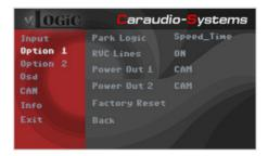
**Exception**: Connect the white wire of harness V6C-NAC01 to analogue rear gear signal (+12V) and make the menu setting - Option 2 / Cam Trigger - "Analogue", if the system doesn't switch to the aftermarket rear-view camera automatically after the described OSD-setup (Option 2 / Cam Trigger - "CAN", see next chapter).
