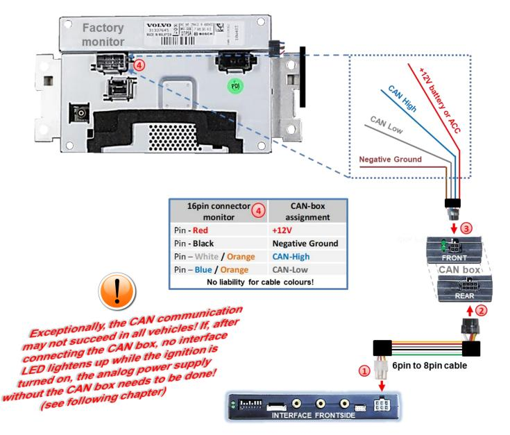
Connect the 6pin to 8pin cable's white female 6pin connector to the male 6pin connector of the video interface.
