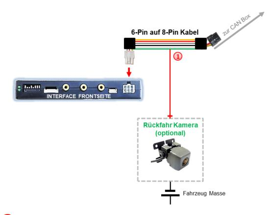
Additionally, the +12V (max. 500mA) power supply for the rear-view camera can be taken from the green wire of the 6pin to 8pin cable.
