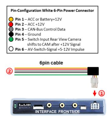
Connect the female 6pin connector of the 6pin to 8pin cable to the 6pin connector of the video interface.
