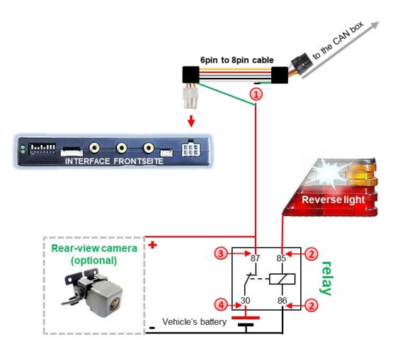
Cut the green cable of the 6pin to 8pin cable close to the black 8pin connector and isolate the shorter end of the green cable near to the 8pin connector (CAN-box side).
