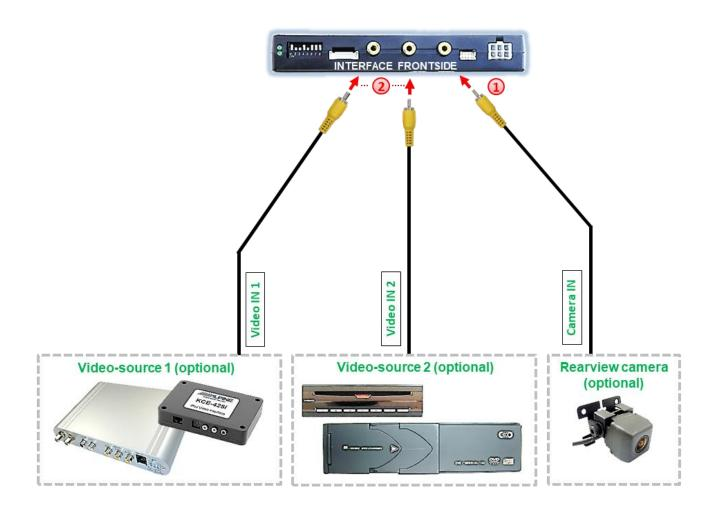
Connect the rear-view camera's male RCA to the video interface's female RCA "Camera IN".
