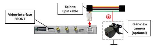
1 Additionally, the +12V (max. 500mA) power supply for the rear-view camera can be taken from the green wire of the 6pin to 8pin cable.
