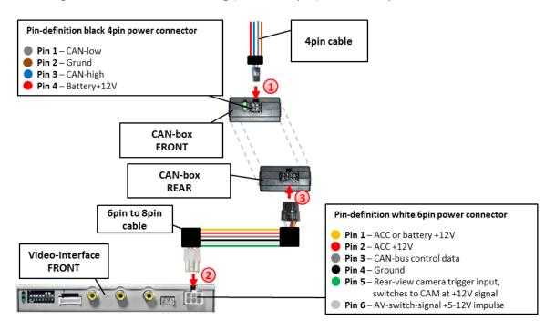
Connect black female 4pin Micro-Fit connector of the 4pin cable to the male 4pin Micro-Fit connector of the CAN-box.
