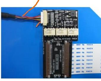
©Solder the Orange wire on NAVI cable to the Head Unit as shown above.
