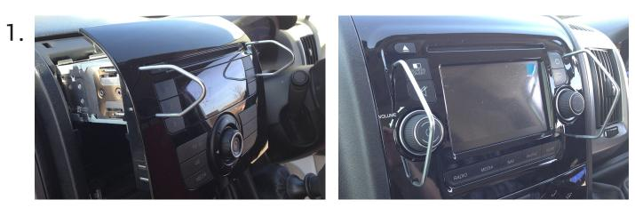
Use a set of release keys to pry the head unit out of the dashboard. Dependent on the style of unit you have installed, you will need either single or double DIN keys. Once released, take out the unit and disconnect all the wiring.
