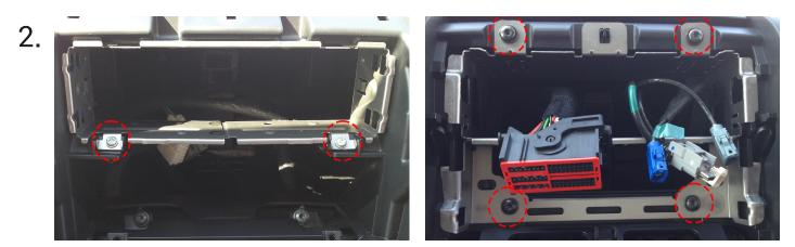
Once the main head unit is out of the way, proceed to remove the highlighted screws. When done, proceed to fully remove the cage.
