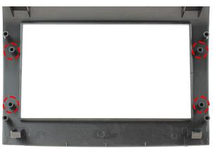
Using the 4x phillips screws, take the brackets and line them up to the following posts on the rear of the new fascia panel and proceed to attach them to the relevant side.
