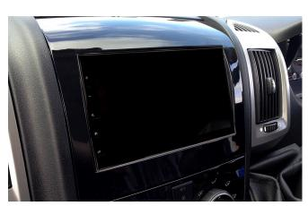
Once the kit has been assembled and the wiring for the stereo is completed, simply use the clips within the kit on the reverse of the fascia and proceed to clip it into place.
