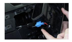
3. Unscrew x2 screws on top of the head unit making sure you only unscrew the screws half way then push the screws down. This will unlock the head unit's bracket assembly.
