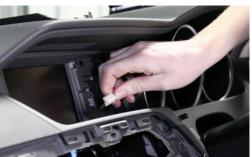
11. Connect to the two brackets on both sides of the display screen by pushing the brackets outwards from the display.
