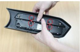
**15.** Place the button panel assembly in front of the display screen. Screw the panel into place – Screws highlighted in the picture, then push the rubber mat into position.
