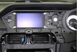
**10.** Connect the extension cable to the white OEM connector that was unplugged from the head unit's fascia panel. Feed the cable up through the dash so the white connector comes out to the right side of the display screen.
