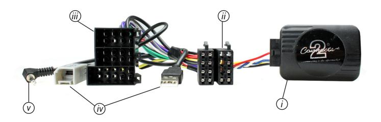
i. Interface Box ii. ISO Connector (16 Pin) iii. Mini ISO Connector iv. USB Male/Female Connectors
