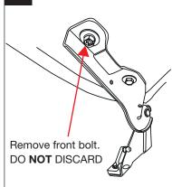
Secure bracket using existing bolt.
