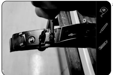
Remove the OEM Rails with Ditch Trim from the vehicles roof by unbolting the nut on the inside of the roof.
