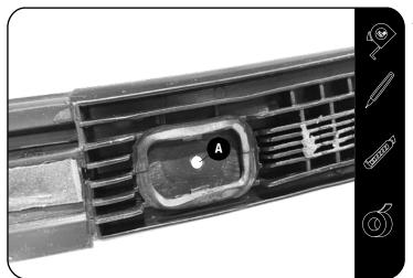
Peel back the weather strip enough so that you can remove the weather strip retaining bolt, Remove the Stud insert from the plastic trim and place the Bottom Spacer (Item 9) into the opening and mark the center of the hole (A).
