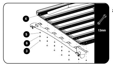
Fit your roof rack to the Foot Rails using M8 x 20 Hex Bolts, M8 x 16 x 1.6 Flat Washers and M8 Nyloc Nuts (Items 4, 5 & 6) as shown.
