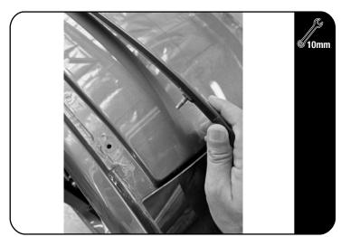
After the Roof Lining is droped, Loosen the M6 nuts on the inside of the Roof holding the Ditch trim in place and remove the Ditch trim from the Roof.
