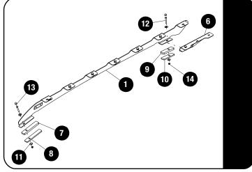
Apply a bead of sealant on the threads of the M6 x 40 Hex Bolts and secure the Foot Rail (Item 1) together with the Support Bracket (Item 6) and the Front and Rear Spacers (Item 7,8 & 9,10) to the Roof using M6 x 40 Hex Head Bolts, M6 x 20 x 2 Flat Washers and M6 Nyloc Nuts (Items 12,13 & 14).
