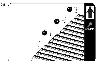
With the Help of a friend lift the Roof Rack on to the roof and place onto the spacers.
