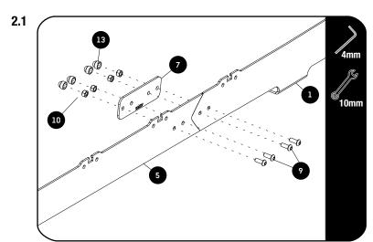
Assemble the Front and Rear Foot Rail (Items 1 & 5) with the Joiner Plate (Item 7) using M6 x 16 Button Head Bolts and M6 Nyloc Nuts (Items 9 & 10) as shown.
