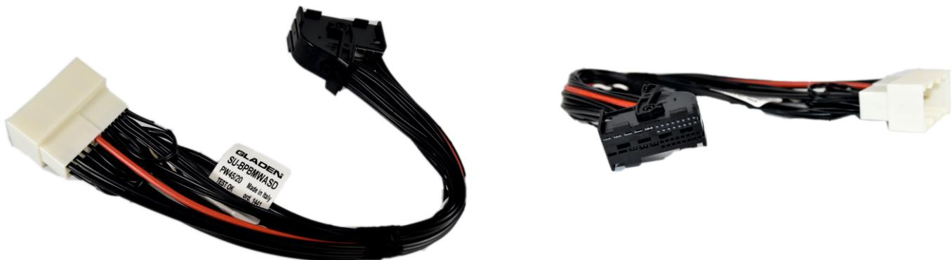
vehicle specific cable set for BMW F/G series with ASD module to bypass the original ASD module
