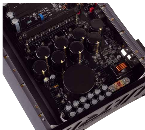
Each channel has its own 50A fuse and a shielded transformer. Rail capacitors are custom made by Mundorf
