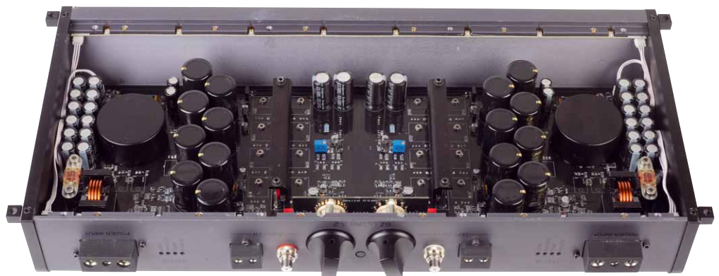
The two channels are totally symmetrical on the PCB, thus achieving the highest possible signal fidelity
