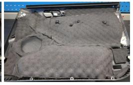
Step 10: Re-assemble the door trim and check the functions of the power window and switches
