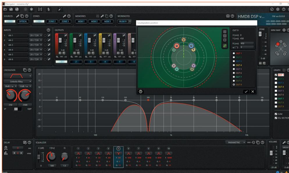
The software was designed to be adopted by all products with onboard DSP in the Hertz marine catalog and future ones: when you connect the device to the software, it automatically configures itself to display the interface of that specific device connected. Navigator can also be used without a real physical device, as it provides a series of virtual devices that fully reflect the respective real counterparts.
