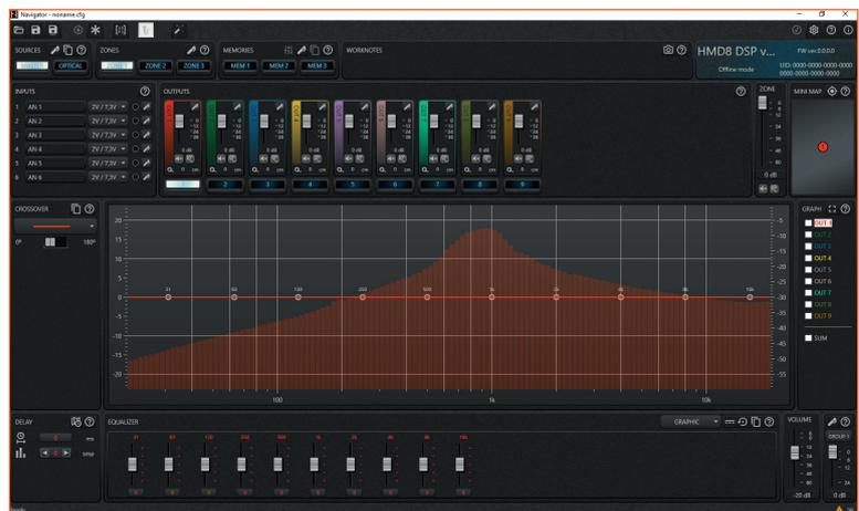
**Remark:** when the RTA function is activated, the audio settings icon is disabled. To change the audio settings it is necessary to turn the RTA off.
