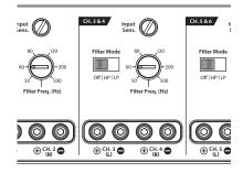
1) "Filter Mode" Control: The M800/8-24V employs a 12dB per octave filter for each pair of channels. Each of these filters can be configured independently into one of two filter types or defeated completely by way of the three-position "Filter Mode" switches:
