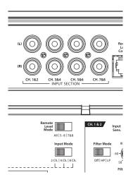
If you wish to send eight discrete channels into the M800/8-24V, simply use all eight inputs and set the "Input Mode" switch in the "8 Ch." position.
