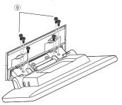
8 Attach the protective cover (accessory (10)) to coupling part, and then fix it with two binding head screws (accessory (11)).
