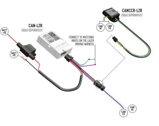
For vehicles where it is not possible to locate a 12V high beam signal, it will be necessary to take the high beam signal from the vehicle's CAN system. For vehicle specific CAN instructions, please download the "CANM8 Cannect" App.
