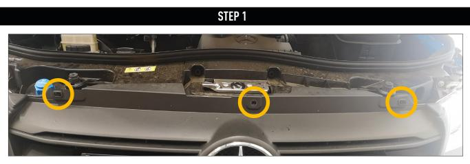
Remove the 3x Screws holding in the grille, and remove the front grille.
