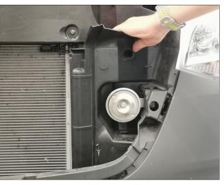
Remove cover's on both sides that are located behind the grille.
