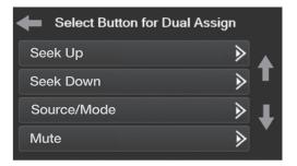
The interface has the capability to assign two functions to a single button, except Volume-Up and Volume-Down. Follow the prompts on the touchscreen display to program the button(s) to your liking.
