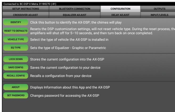
**RESET TO DEFAULTS:** Resets the interface to factory settings. During the reset process the amplifiers will shut off for 5-10 seconds.
