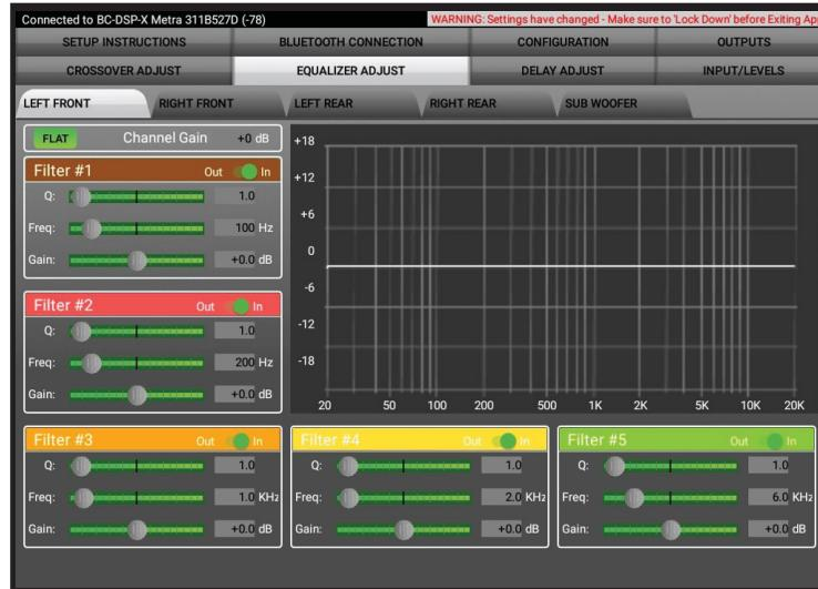
Each output has a **5 Band parametric EQ** per channel. Each band will give the user the ability to adjust:
