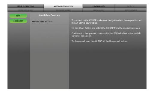
Scan - Press this button to start the Bluetooth pairing process, then select the interface
