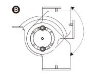
A. RECOMMENDED GUIDE LINE FOR ASSEMBLING SUNSHIELD. B. USER CAN ADJUST THE INSTALLING ANGLE
