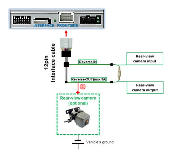
The 12 V power supply for the rear-view camera (max 3A) has to be taken from the 12pin interface cabl's green wire "Reverse-OUT" to avoid an unnecessary, permanent power supply to the camera electronic.
