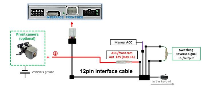
1 The red power supply output ACC/front cam out 12V (max 3A) can be used to power a front camera. If Dip 1 is set to ON (black 8 dips), the power supply output gives +12V (max 3A) when reverse gear is engaged incl. 10 seconds delay after reverse gear is disengaged.
