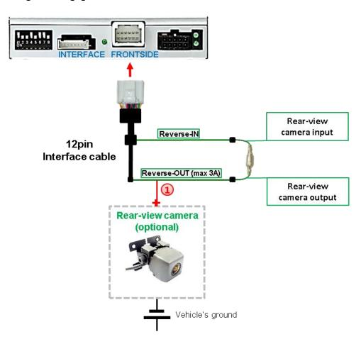
1 The 12 V power supply for the rear-view camera (max 3A) has to be taken from the green wire of the 12pin interface cable to avoid an unnecessary, permanent power supply to the camera electronic.
