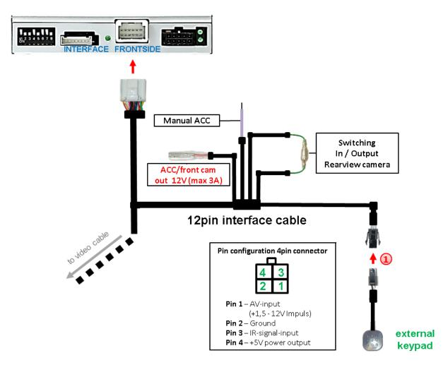
Connect the female 4pin connector of the keypad to the male 4pin connector of the 20pin interface cable.
