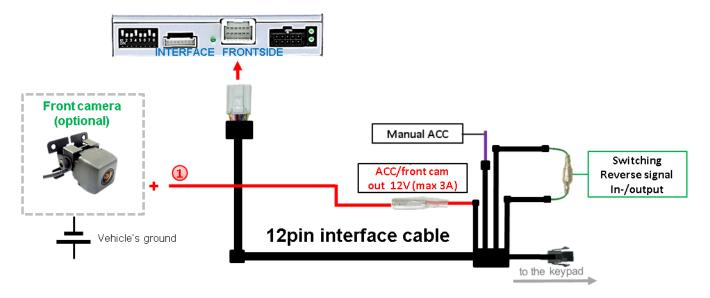
1 The red power supply output ACC/front cam out 12V (max 3A) can be used to power a front camera. If Dip 1 of the black 8 dips is set to ON, the power supply output gives +12V (max 3A) when reverse gear is engaged incl. 10 seconds delay after reverse gear is disengaged.
