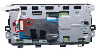
Clip the shorter 60pin ribbon cable coming from the mainboard into the input (CAR\_IN) of the daughter PCB and the longer twisted 60pin ribbon cable going to the monitor panel into the output (PNL OUT) of the daughter PCB.
