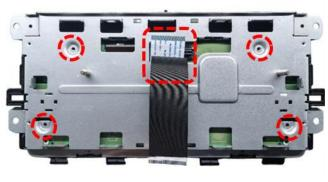
Carefully fold the mainboard back. Clip the 2 OEM ribbon cables coming from the monitor panel back onto the mainboard and plug the small white male connector back in.
