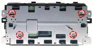
Unscrew the 4 screws on the back of the head unit and remove the housing cover.
