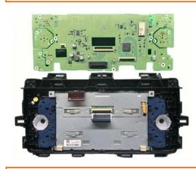
Unclip the 3 OEM ribbon cables coming from the monitor panel on the mainboard and disconnect the small white male connector.
