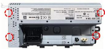
Replace the housing cover, ensuring that the 20-pin picture signal cable is routed out of the side.
