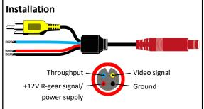
Note: If the camera is powered by reverse gear lamp signal, we recommend to install a relay between the power supply of the reverse signal and the power supply of the camera, to ensure a stable and uninterrupted power supply and to avoid vehicle computer errors. The throughput wire can be used to connect the reverse gear lamp signal from back to front.
