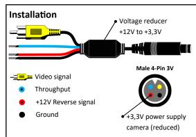
**Note:** If the camera is powered by reverse gear lamp signal, we recommend to install a relay between the power supply of the reverse signal and the power supply of the camera, to ensure a stable and uninterrupted power supply and to avoid errors in the vehicle computer.
