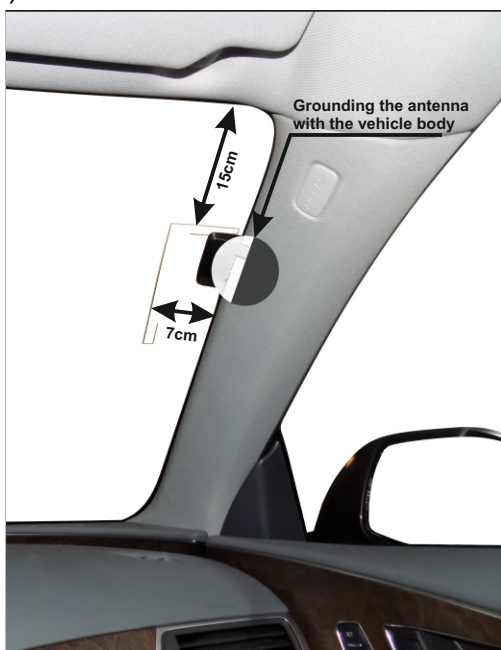
Example of mounting a DAB/DAB+ antenna
